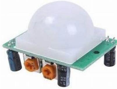
**Gambar 1.** Sensor Passive Infrared Receiver
