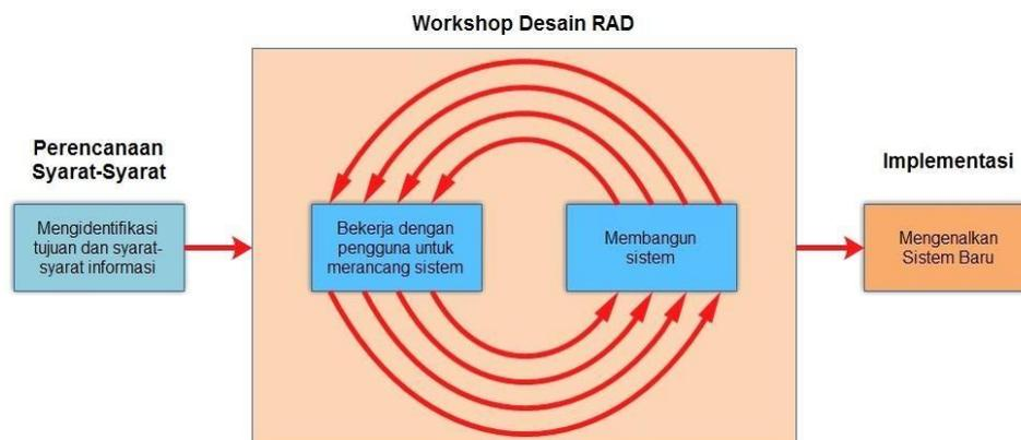
Gambar 1. Tahapan Metode Rapid Application Development (RAD)
